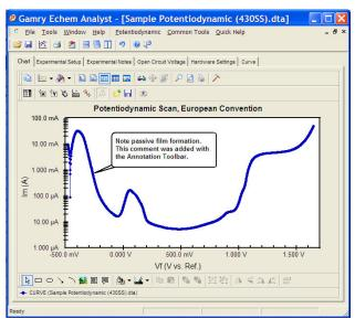
**Potentiodynamic Scan.** This Potentiodynamic Scan is plotted with the European convention of log current on the Y-axis. The plotting format can be easily reversed if you prefer. Note the annotation and the Annotation Toolbar on the bottom.
