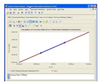
*A Polarization Resistance Experiment Displayed in the Echem Analyst.* The dark blue curve segment is used to calculate the corrosion rate. Note the Corrosion Rate on the lower portion of the display. More detail is available on the PolRes tab.
